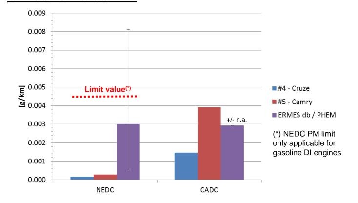
• Measured vehicles show typical low PM levels of gasoline engines
