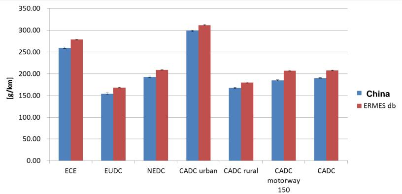
→ On average China results 8% lower (min: -4% in CADC urban; max: -11% in CADC motorway) 中国平均测试结果较ERMES低8%
