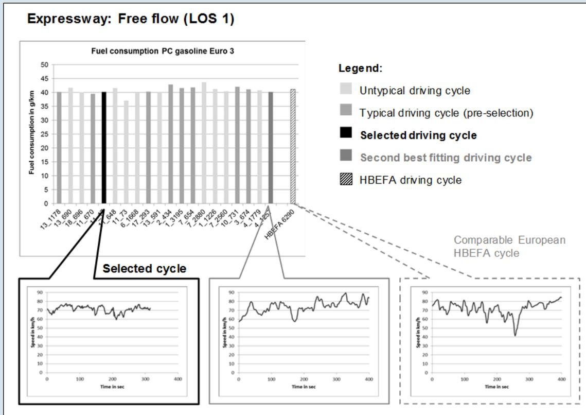
**Figure 10: Selection of the typical traffic situation for passenger cars for the traffic situation “Expressway”: Free flow based on the top 20 cycles selected for Beijing and Shenzhen**
