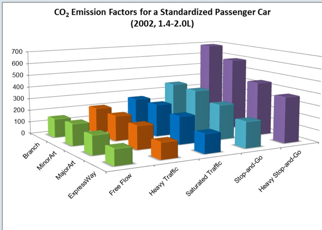
**Figure 11: CO<sub>2</sub> emission of a standardised passenger car (construction year 2002, engine capacity 1.4 - 2.0 l) for Chinese traffic situations**
