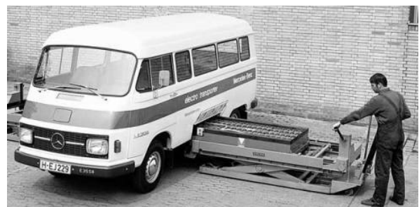
Figure 2: Battery swapping on an electric Mercedes bus in the 1970s, Source: The Green Optimistic
