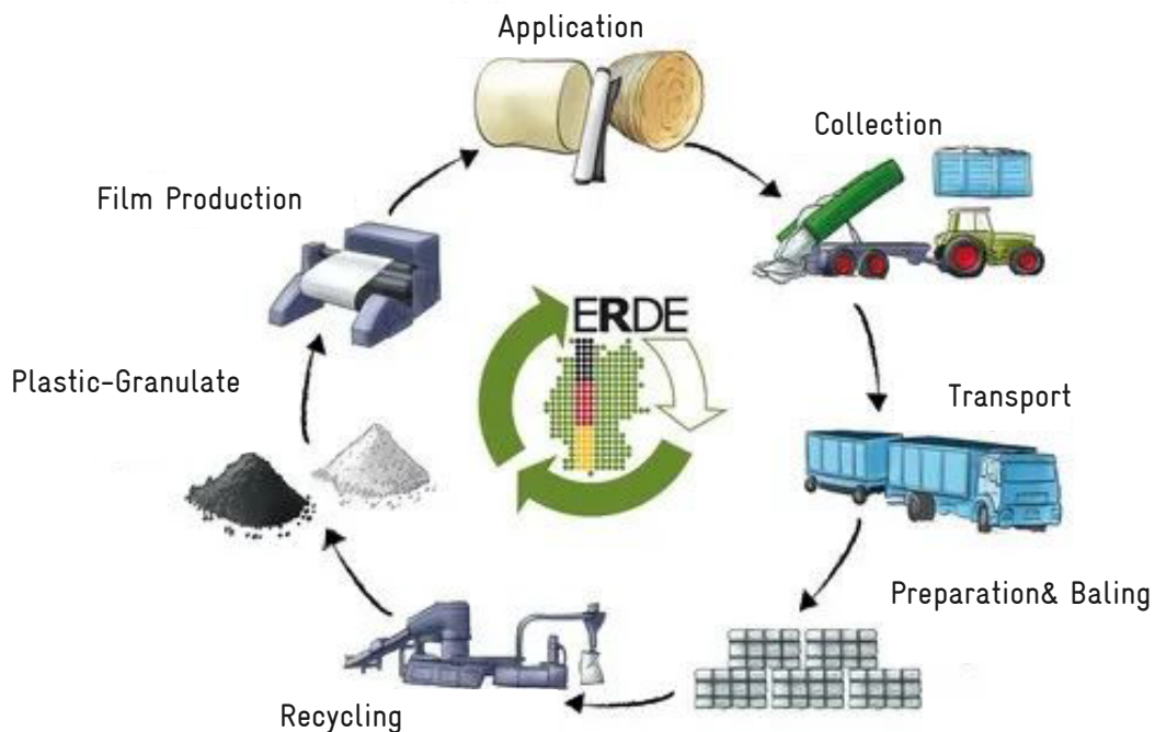
Figure 23 Agricultural plastic recycling system of ERDE in Germany
