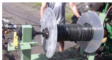
Figure 19 Irrigation pipe collection in Florida, USA
